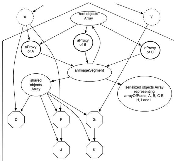
Figure 3: Objects state after the ImageSegment extraction
