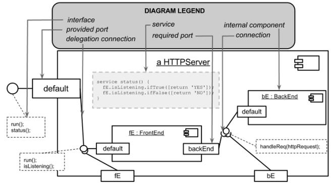
**Figure 2: Diagram of an HTTPServer component instance**
