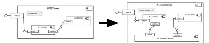
Figure 3: Simplified diagram illustrating the transformation from classic front-end back-end architecture into bus-oriented architecture.
